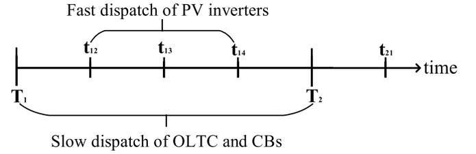
Fig. 1. Multi-timescale voltage regulation framework in VVO.
