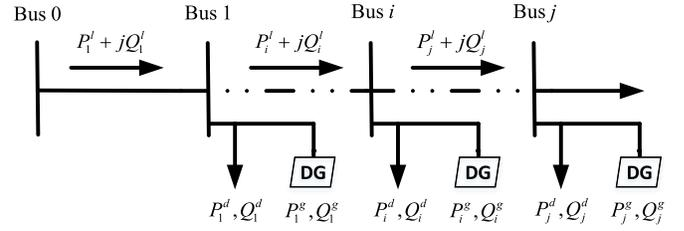
Fig. 2. Schematic diagram of a radial distribution system.
