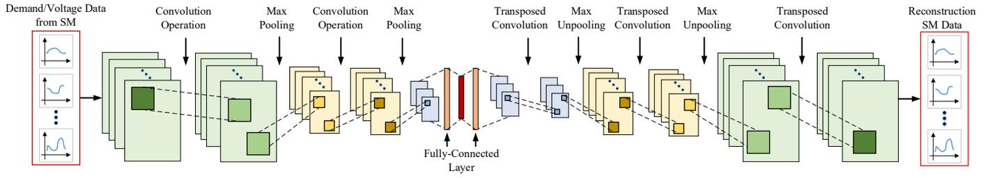
Fig. 2: DCA-based SM data compression and reconstruction.
