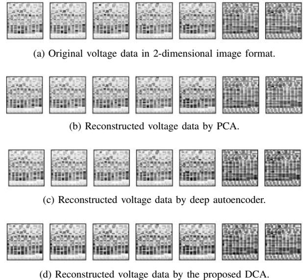
Fig. 5: Comparison of voltage data compression results.
