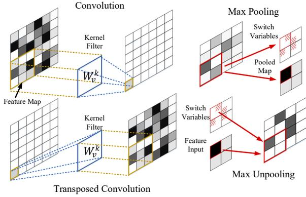
Fig. 3: Illustration of convolution, max pooling, transposed convolution, and max unpooling.
